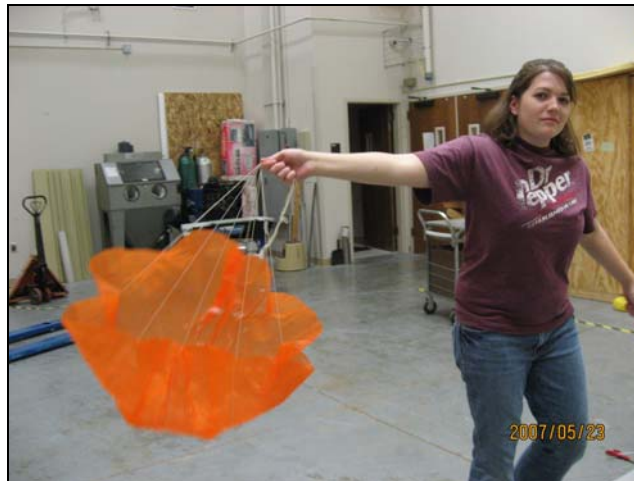
Figure 13 - Fluff out parachute by swiftly pulling it behind you
